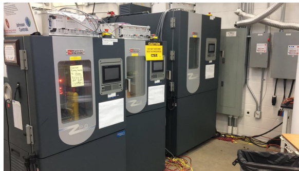
Figure 2.2: Battery test chambers that housed the physicals cells during battery tests to keep temperature controlled
