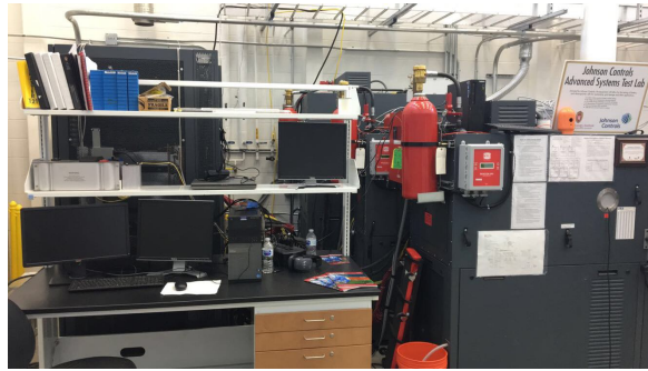
Figure 2.1: Front view fo the test station used to control the Digatron system to perform battery tests
